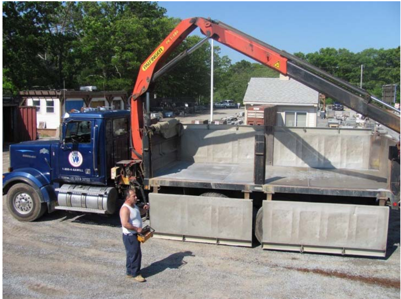
1998 WESTERN STAR F850 Triaxle, Cat (C-12) 9NS04915 8LL spd. trans, AC, Tires 385/65R22.5, Rear axle 46,000. lbs, Palfinger PK14080 27' Boom, Showing side doors & rear dump with scuttle, overall length 32' Well Maintained..... $25,000. or B.O.
